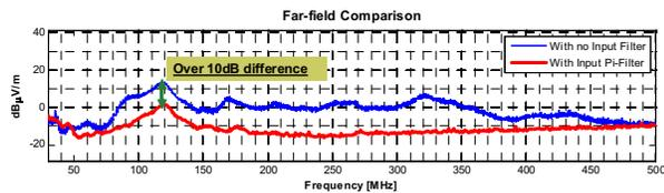
Figure 12. Impact of Adding an Input Filter on Far-field Broadband Noise
