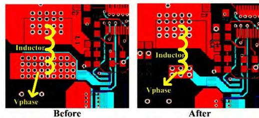
Figure 14. Reducing the Size of the Exposed Phase Voltage Plane
