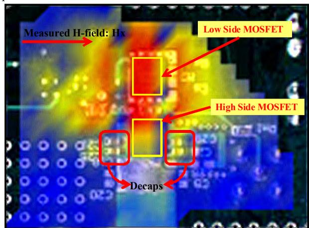
Figure 15. Magnetic Field around Switching Loop (Help of Amber Precision Instruments – [www.amberpi.com](http://www.amberpi.com))
