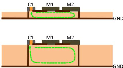
Figure 8. Dielectric Thickness
