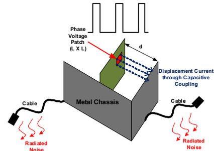
Figure 13. Electric Coupling from Exposed Phase Voltage Plane
