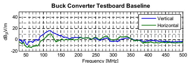
Figure 2. Far-field EMI from Synchronous Buck Converter Test Board
