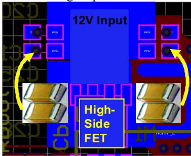
Figure 6. Capacitor Placement Experiment
