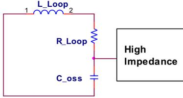
Figure 4. Switching Loop (Top) and the Equivalent Model when High-side MOSFET is on and Low-side MOSFET is off
