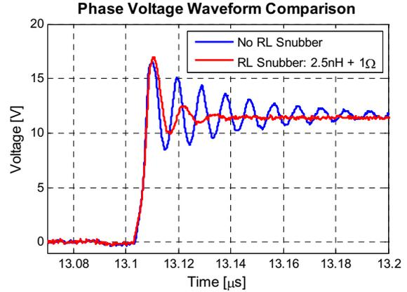
Figure 14. Phase Voltage Comparison with RL Snubber
