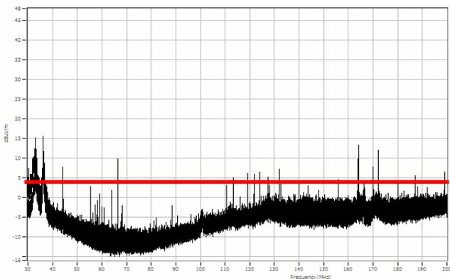
Figure 8. X2Y Filter board implemented and attached to Amphenol connector of test box. The figure below shows the improved radiated emissions performance
