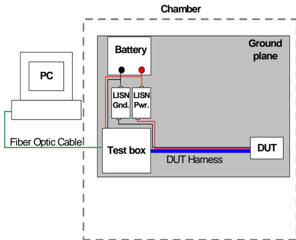
Figure 1. Generic test setup for EMC testing
