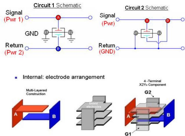
Figure 7. X2Y capacitor circuit configurations and physical structure
