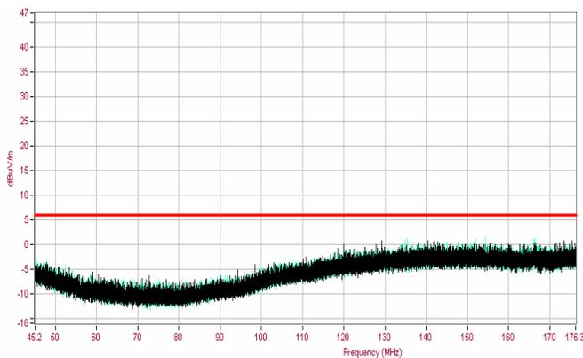
Figure 5. Simple lighting test box with traditional filtering & improved radiated emissions performance.
