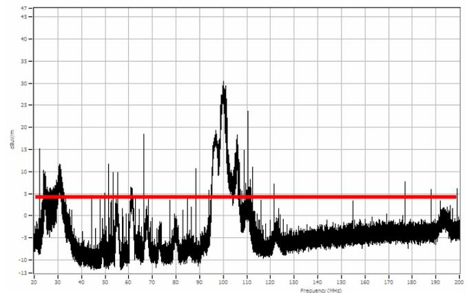
Figure 6. Complex Telematics tester with traditional filtering & moderately improved radiated emissions performance
