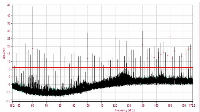
Figure 2. Lighting Test box – without filtering & CISPR 25 Radiated Emissions results for the unmodified lighting test box
