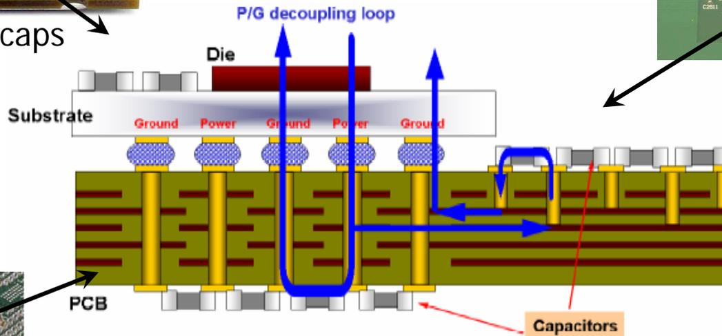
Fig. 1. System decoupling loops for PCB-mounted decoupling capacitors.
