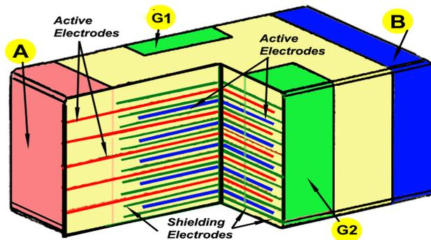
Figure 9. X2Y® Shielding Electrode Architecture
