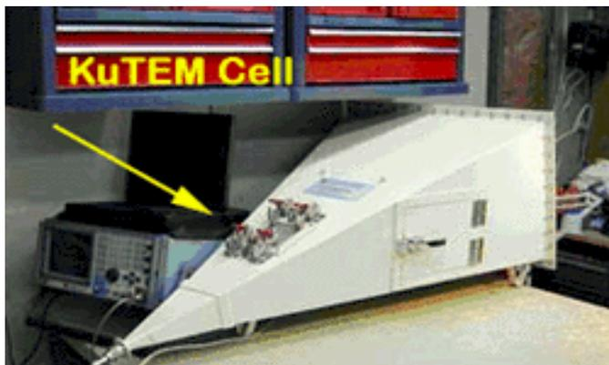
**Figure 2.** A KuTEM Omni-Cell with Spectrum Analyzer.
