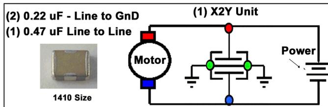
Figure 8. (1) Component Motor Filter Unit.
