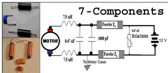
Figure 6. (7) Component Motor Filter Network.
