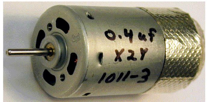
**Figure 3.** DUT shown with Tin-plated Copper Foil Tape Applied
