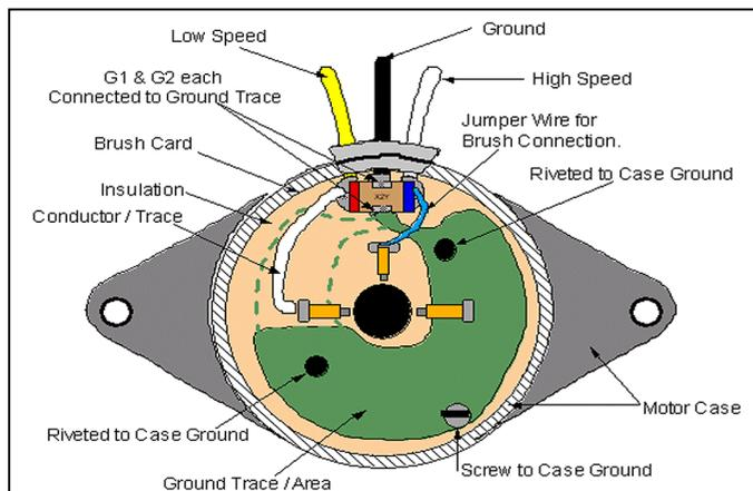
Figure 13. Typical X2Y placement inside a DC Motor
