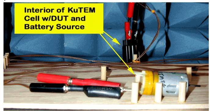
**Figure 4.** Baseline DUT shown inside KuTEM Omni-Cell
