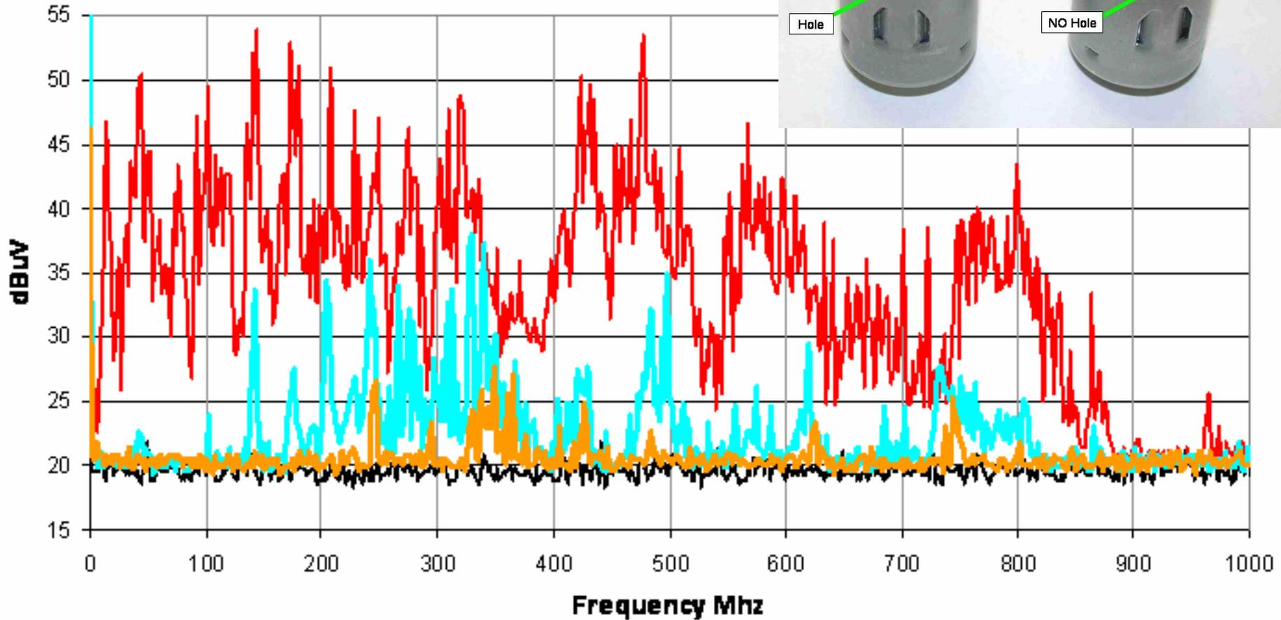
— Ambient — No Filter — X2Y Motor - 0.44 uF — X2Y Motor - 0.44 uF w/ No Holes Near Brushes
