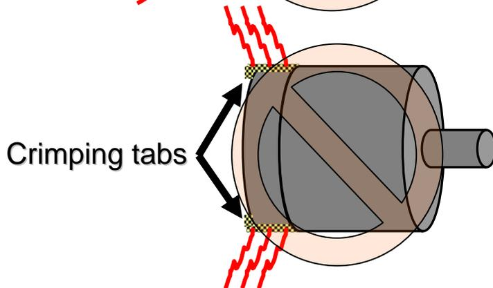
A metal end cap works as a shield to contain the noise within the motor case.
