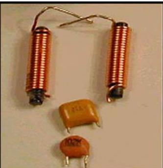
**Capacitor + (2) Inductors + Capacitor**
