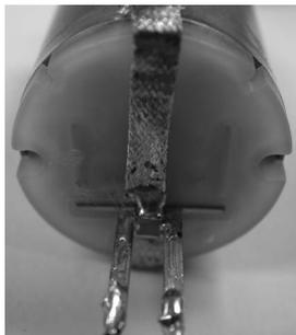
Figure 12. X2Y<sup>®</sup> component prototyped on the outside of the washer-pump. (Note: the prototyped motor used a 1014 size X2Y<sup>®</sup> for easier attachment).
