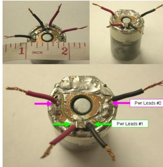
**Figure 1.** Prototype DC motor with two placements for power leads.
