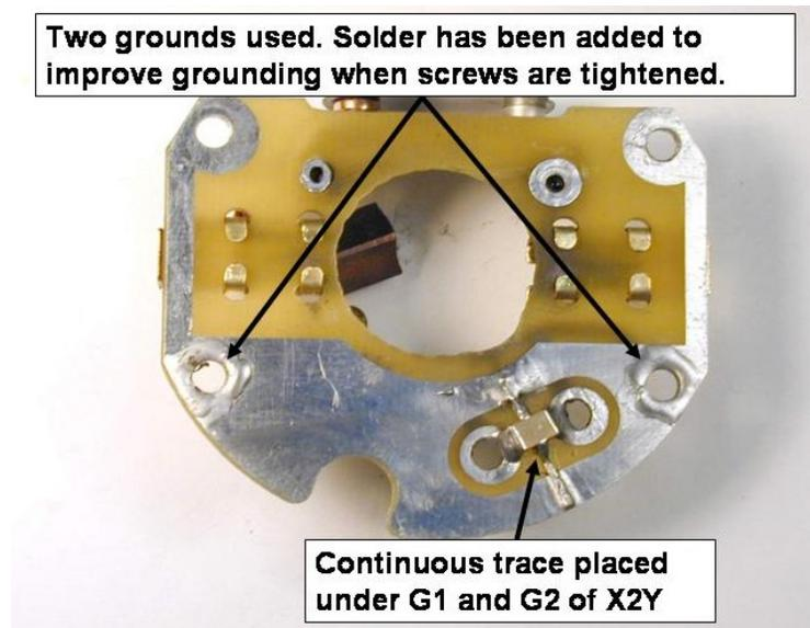
**Figure 4.** *Mock-up to fix design issues.*
