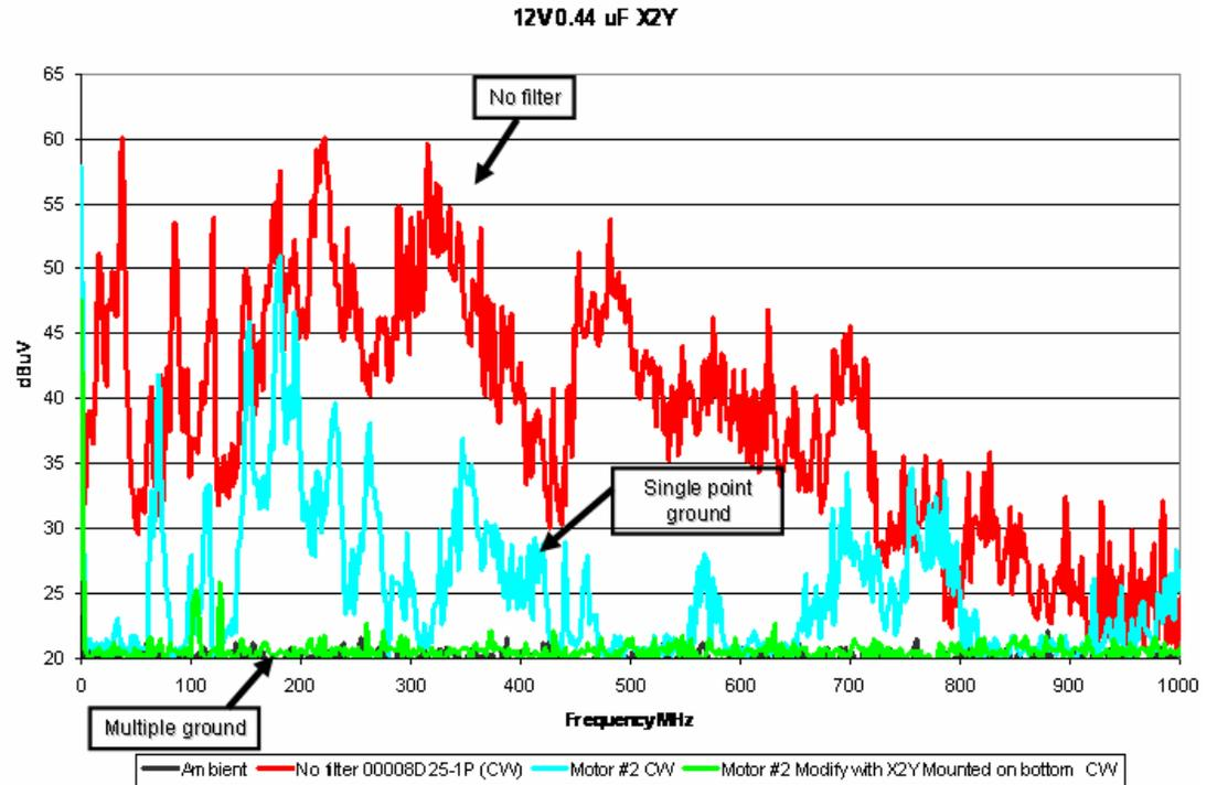
**Figure 5.** Radiated emissions test results.
