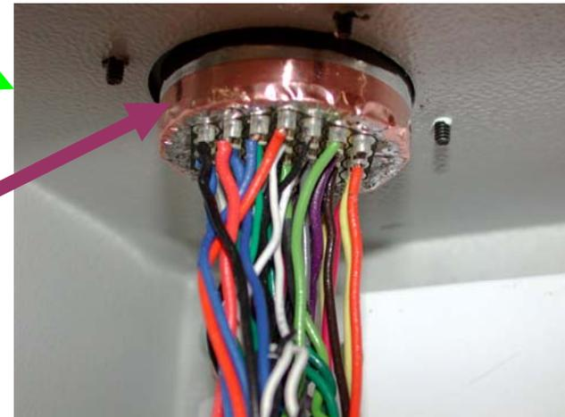
Non-conductive coating removed behind connector
