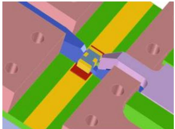
A midsection is inserted into the Test Fixture. The size of the midsection determines the size of the DUT to be tested. The midsection assembly has 2 guide holes for alignment with the test fixture. The chamfered side of the alignment holes are towards the input side of the test fixture on all midsections.
