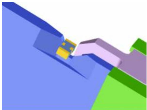
2 DUT guides help place the DUT evenly onto the RF-contacts (DUT guides are shown in blue).
