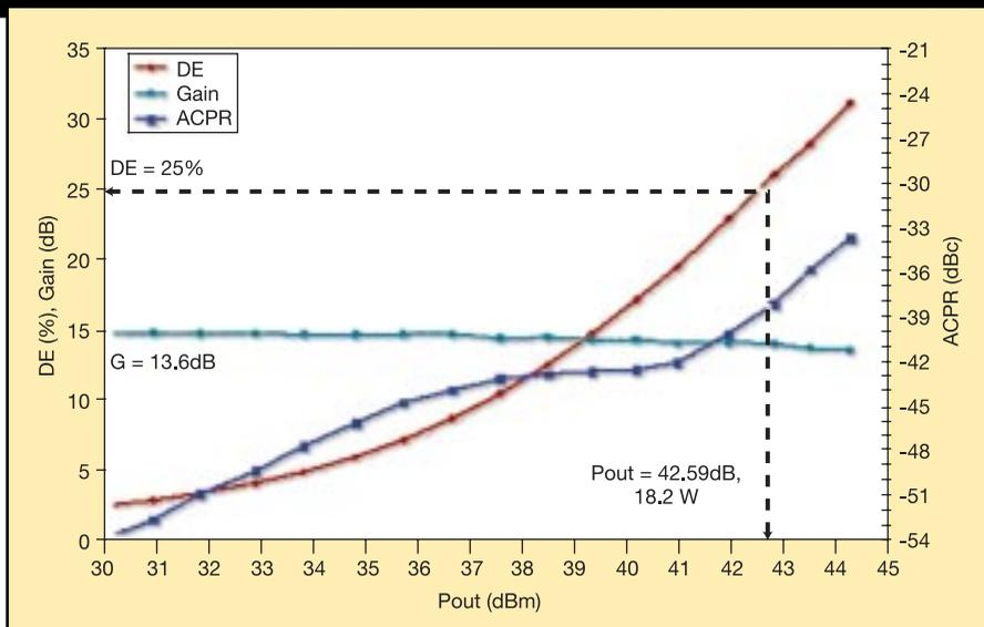
**Figure 2.** Nitronex's 2.14 GaN HFET, NPT2110, offers 18.2 W power at 25% efficiency with a gain of 13.6 dB.
