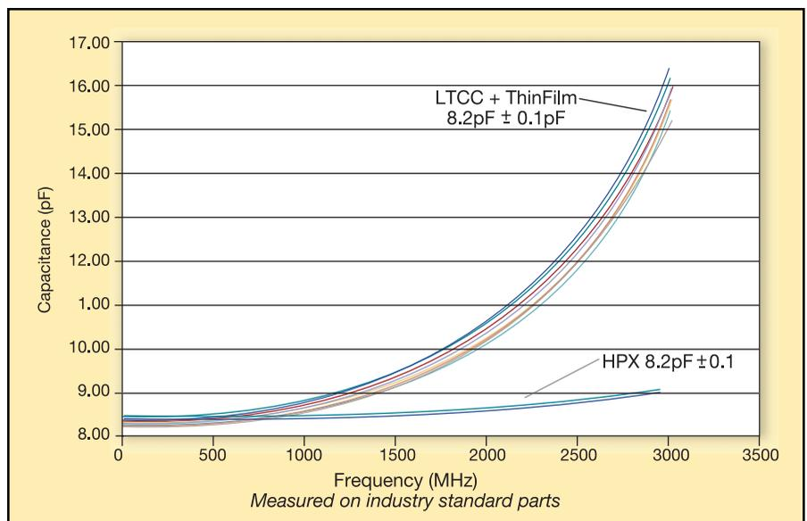
**Figure 3.** Performance of low temperature, co-fired ceramic (LTCC) vs. discrete high precision capacitor. Courtesy of Vishay Intertechnology.
