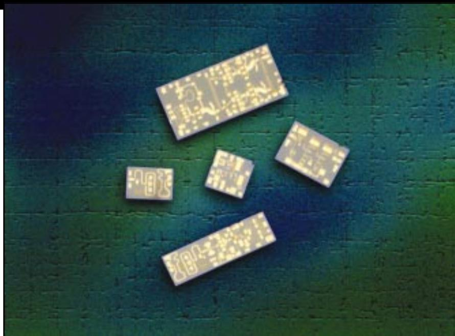
Figure 4. Agilent's newest LNA, AMMC6241, is rated from 26 GHz to 43 GHz with a gain of 20 dB and a noise figure of 2.7 dB.
