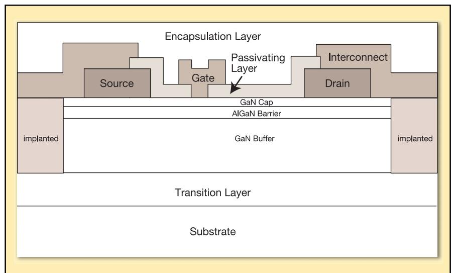
Figure 1. Cross-section of GaN heterostructure FET (HFET).
