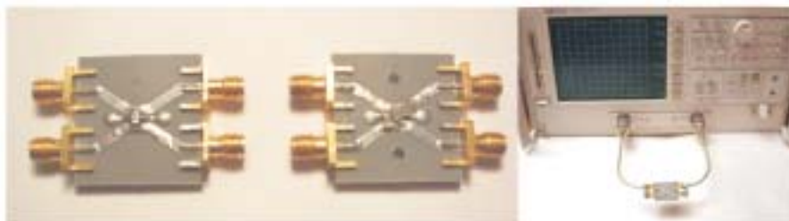
Figure 8. Printed circuit board test fixtures, attached to vector network analyzer.
