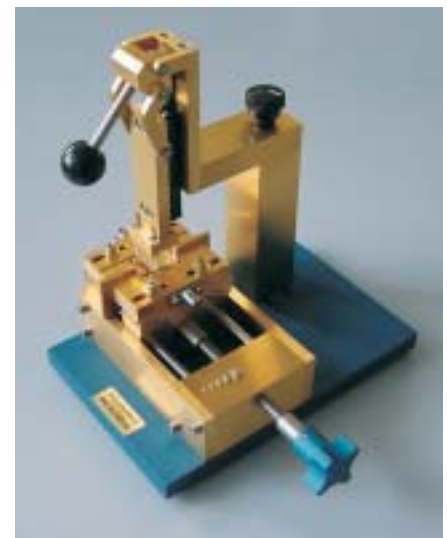
Figure 11. ICM four terminal surface mount test fixture. 12
