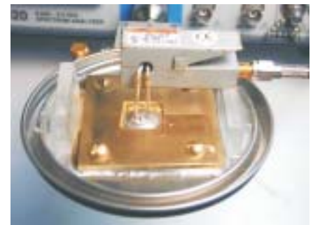
Figure 5. Dual-line test jig.
