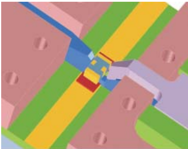
Figure 13. Midsection in fixture for DUT measurement.
