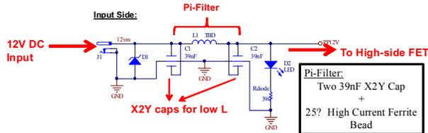
Figure 11. Input Pi-filter for Filtering High-frequency Noise on the DC Input Rail
