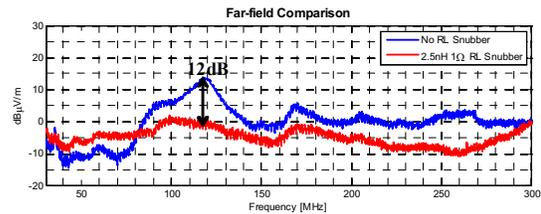
Figure 15. Far-field Noise Comparison with RL Snubber
