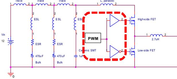
Figure 3. Input and Switching Cell Part of the Synchronous Buck Converter with Parasitic Inductances
