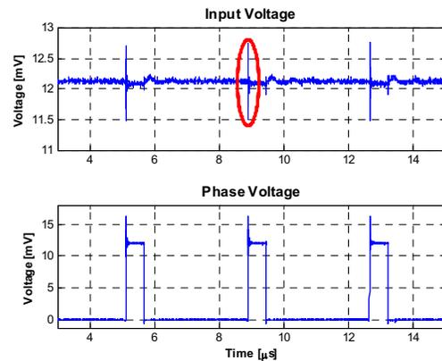
Figure 10. High Frequency Noise on the 12V Rail
