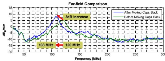
Figure 7. Impact of Input Decoupling Capacitor Placement on Radiated Broadband Noise
