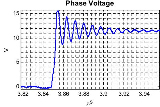
Figure 5. Ringing in the Phase Voltage Waveform Due to Parasitic Resonance in the Switching Loop
