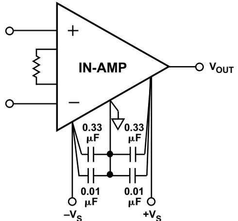
Figure 5-1. Recommended Method for Power Supply Bypassing
