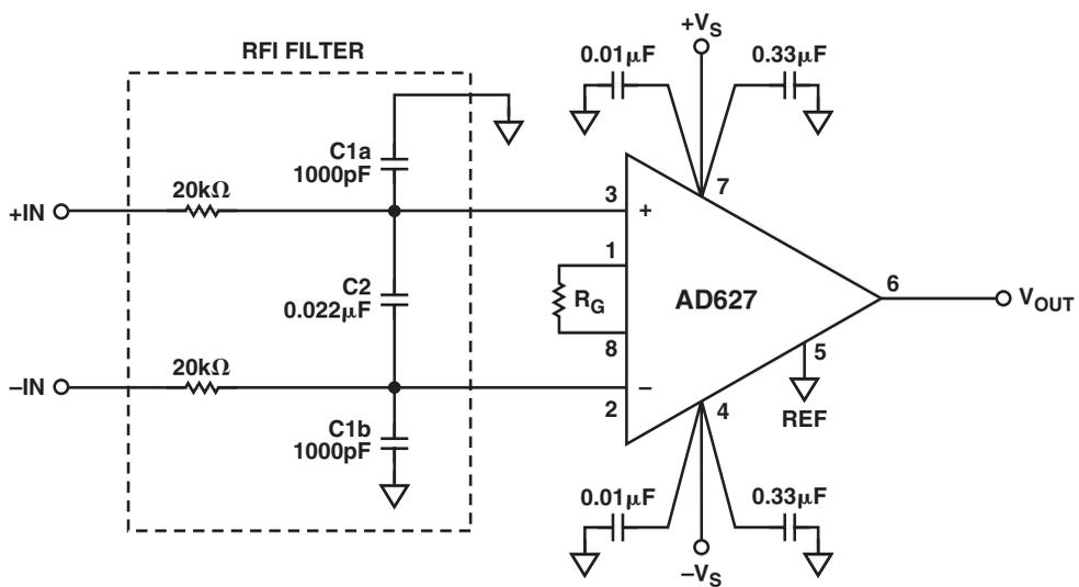
Figure 5-16. RFI Suppression Circuit for the AD627
