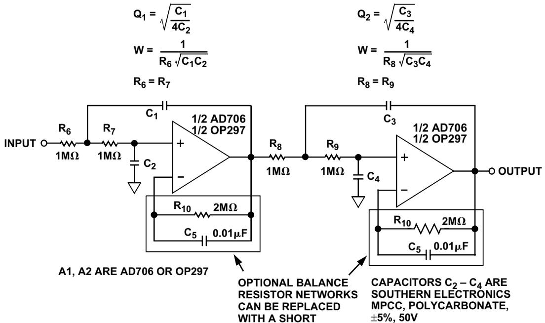
Figure 5-24. A 4-Pole Low-Pass Filter for Data Acquisition
