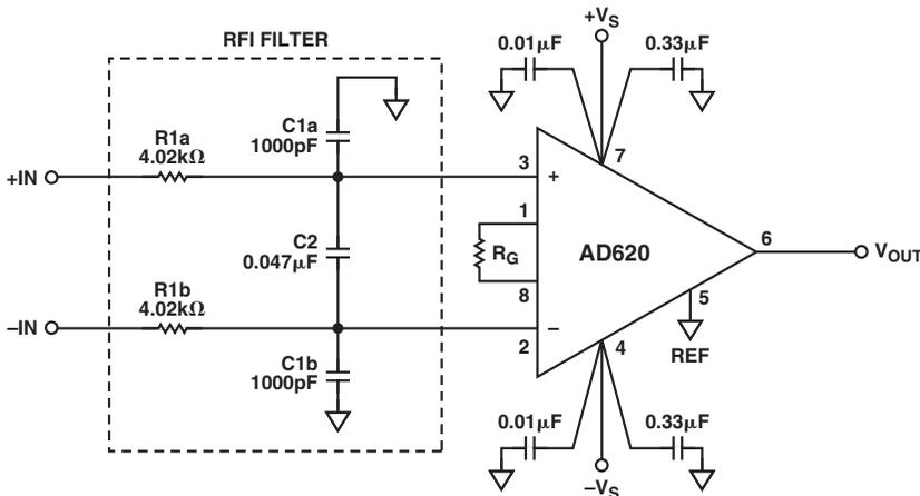
Figure 5-15. RFI Circuit for AD620 Series In-Amp
