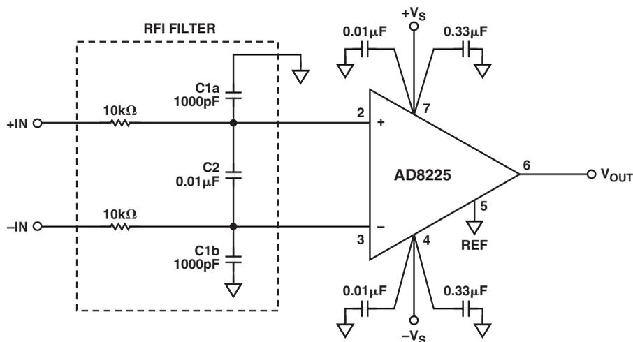
Figure 5-18. AD8225 RFI Filter Circuit
