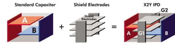
Fig. 1: Construction of the X2Y IPD
