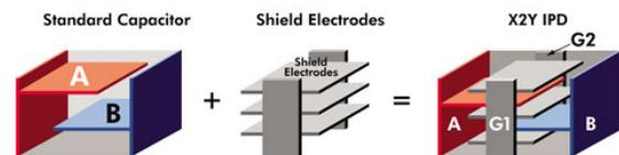
Fig. 1: Construction of the X2Y IPD
