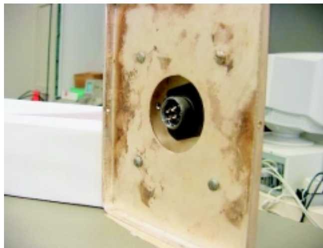
Figure 20. Mounting shield used in test setup.
