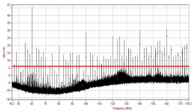
Figure 2. Lighting Test box – without filtering & CISPR 25 Radiated Emissions results for the unmodified lighting test box
