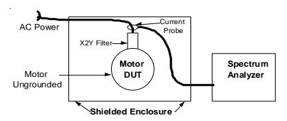
**Test Set Up**
