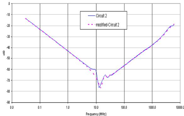
**Figure 8.** S21 plot comparing X2Y<sup>®</sup> Circuit 2 to modified-Circuit 2 configuration. The component used here was a 1210 X2Y<sup>®</sup> 560nF.
