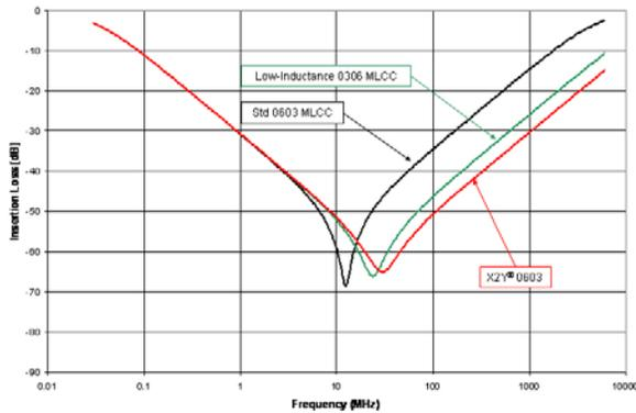
**Figure 10.** S21 plot of standard 0603 MLCC, low-inductance 0306 MLCC, and 0603 X2Y<sup>®</sup> component. Data provided by Bart Bouma of Yageo-Phycomp.
