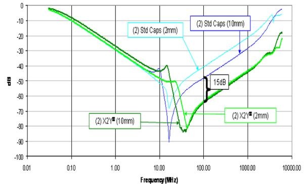
**Figure 9.** S21 plot of (2) standard MLCC versus (2) X2Y<sup>®</sup> components spaced 2mm and 10mm apart.
