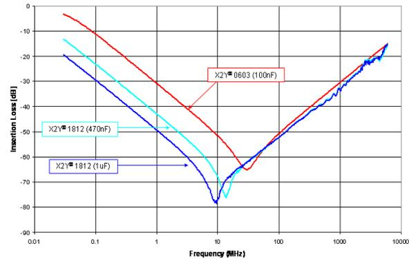
**Figure 11.** S21 plot of 0603 (100nF) X2Y<sup>®</sup>, 1812 (470nF) X2Y<sup>®</sup>, and 1812 (1uF) X2Y<sup>®</sup>. Data provided by Bart Bouma of Yageo-Phycomp.
