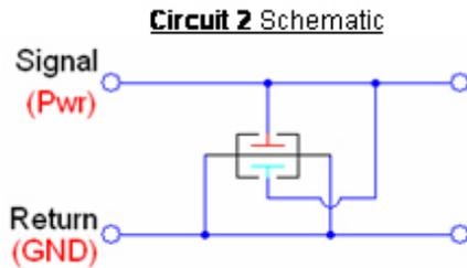
**Figure 4.** Schematic of the X2Y<sup>®</sup> Circuit 2 configuration.
