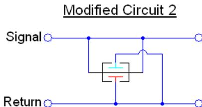
**Figure 7.** Schematic of the X2Y<sup>®</sup> modified-Circuit 2 configuration.
