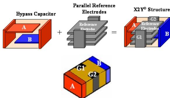
Figure 1. Depiction of the X2Y<sup>®</sup> structure.
