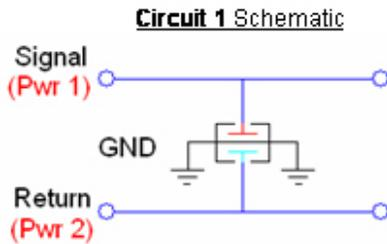
**Figure 3.** Schematic of the X2Y<sup>®</sup> Circuit 1 configuration.
