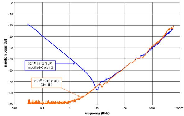
**Figure 12.** S21 plot of X2Y<sup>®</sup> Circuit 1 and Circuit 2 configurations.
