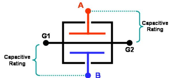
Figure 2. Illustration of the X2Y<sup>®</sup> capacitive rating.
