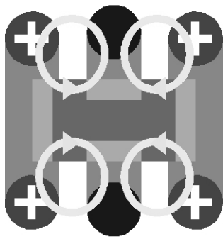
Figure 10, X2Y & Surface Induction Loops
