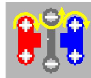
**X2Y<sup>®</sup> Structural Benefit – shorter path to ground, which creates a smaller current loop when attached to the PCB.**
