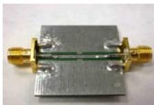
✓ Measurements made on 50ohm Coplanar PCB with Ground Plane.
