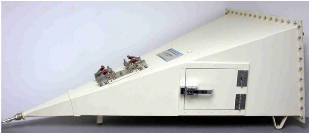
ETS-LINDGREN GTEM Model 5402 [www.emctest.com](http://www.emctest.com)
