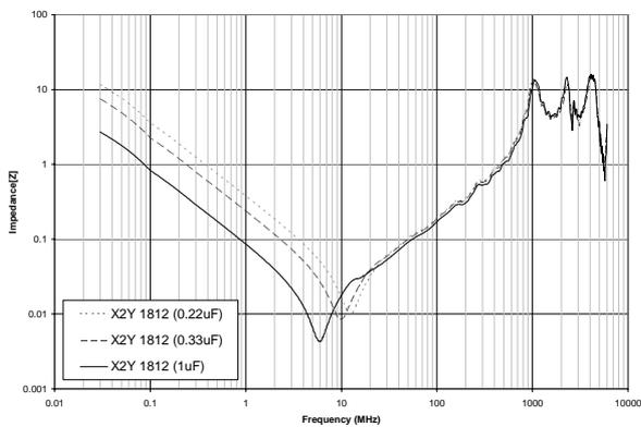
Figure 13. Via-PCB plot comparing different capacitance values.
