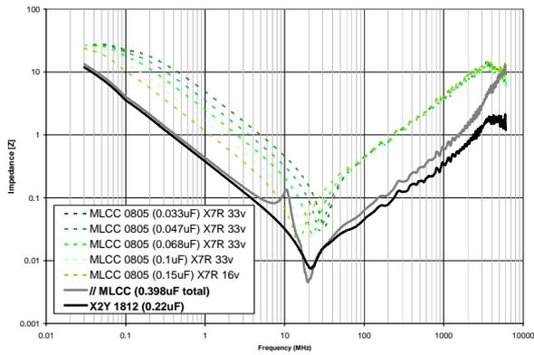
Figure 16. Multiple different value 0805 MLCCs in parallel compared to a single equivalent value 1812 X2Y<sup>®</sup> component.
