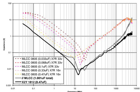
Figure 15. Multiple different value 0805 MLCCs in parallel compared to a single equivalent value 1812 X2Y<sup>®</sup> component.
