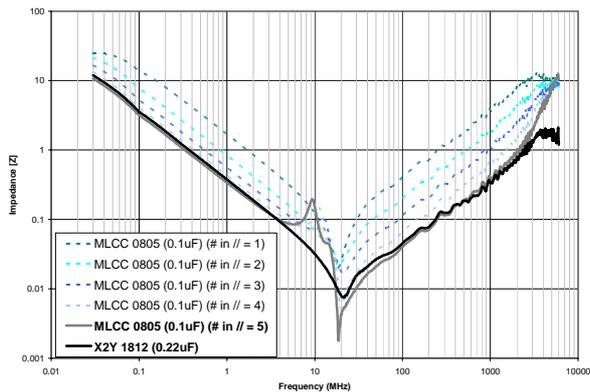
Figure 17. Multiple same value 0805 MLCCs in parallel compared to a single equivalent value 1812 X2Y<sup>®</sup> component.
