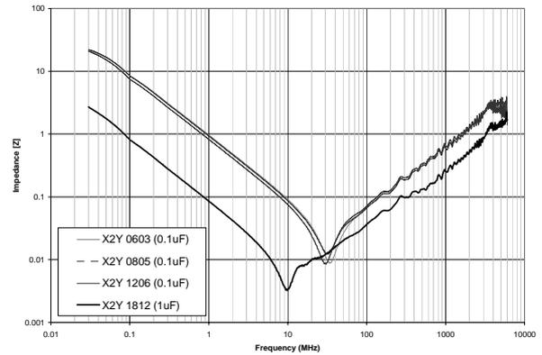
Figure 10. Microstrip-PCB impedance plot comparing different package sizes.
