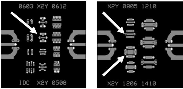
Figure 7. 0603 via-PCB (top-left) & 0805 & 1206 via-PCB (top-right).
