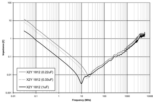
Figure 12. Microstrip-PCB plot comparing different capacitance values.
