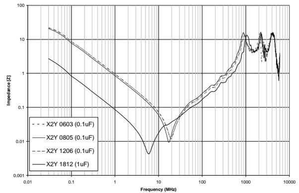
Figure 11. Via-PCB impedance plot comparing different package sizes.
