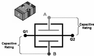
Figure 5. Illustration of X2Y<sup>®</sup> capacitive rating.
