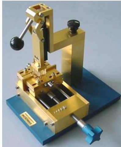
Figure 3. Microwave test fixture used to measure insertion loss. Photo courtesy of Yageo-Phycomp.
