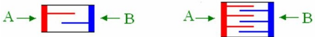
Figure 1. Standard capacitor construction is made up of alternating electrode plates. To increase capacitance value, multiple alternating plates are added.
