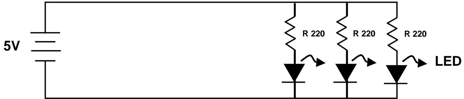
Typical LED circuit with a series limiting resistor <sup>1</sup>
