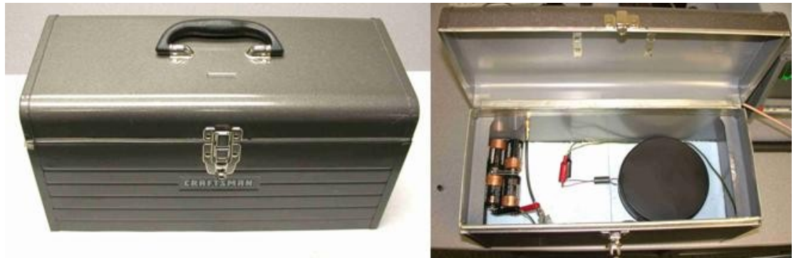
Figure 9. Modified metal toolbox used to measure conducted emissions (left); DUT placement (right).
