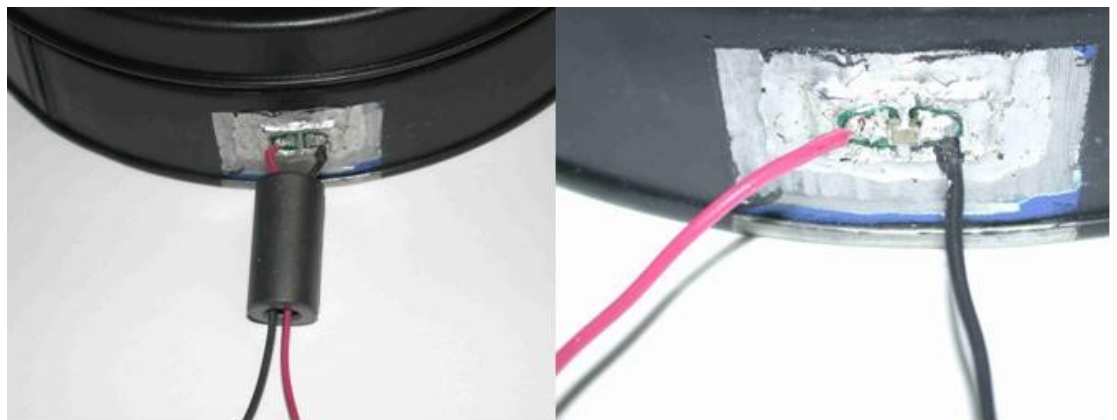
Figure 4. DUT placement on metal enclosure.
