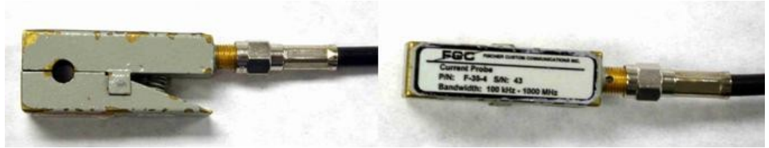
Figure 8. Current Probe (FCC F-35-4).
