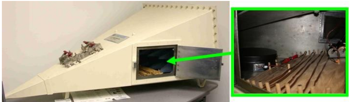
Figure 5. GTEM (ETS-Lindgren IC-GTEM 250) to measure radiated emissions (left); DUT placement in GTEM (right).
