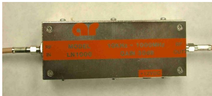
Figure 7. Preamp (AR LN1000) used to amplify the frequencies 200 MHz to 1 GHz.
