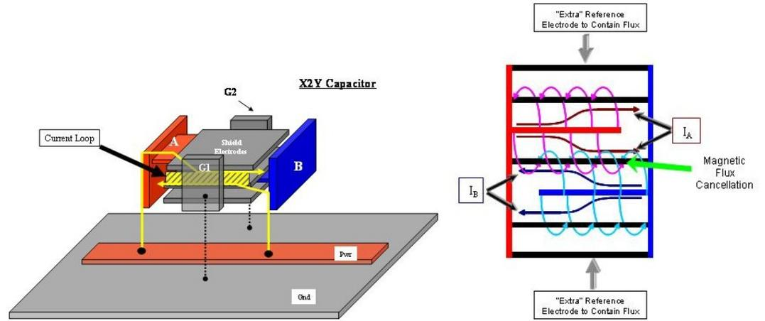
**Figure 6.** X2Y® structure showing opposing currents and magnetic flux cancellation.
