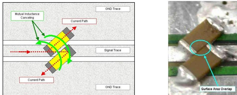
**Figure 5.** *Best-case standard capacitor configuration for cancellation.*
