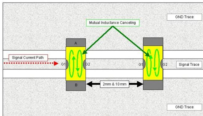
**Figure 9.** X2Y® component configuration for Test #2.
