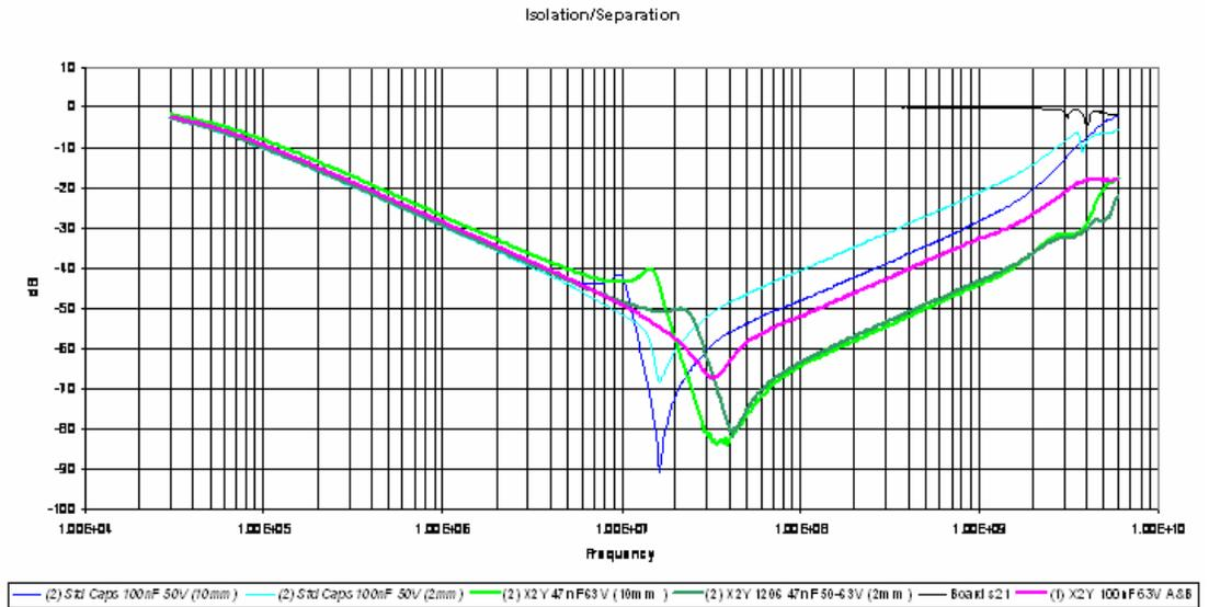
**Figure 10.** s21 measurement results for Test #2 – Isolation/Separation. (Note: All tests in the above figure have equal total capacitive values.)
