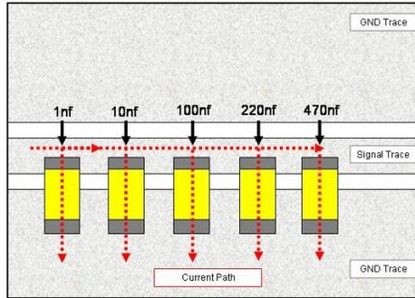
Figure 11. Standard capacitor configuration for Test #3.
