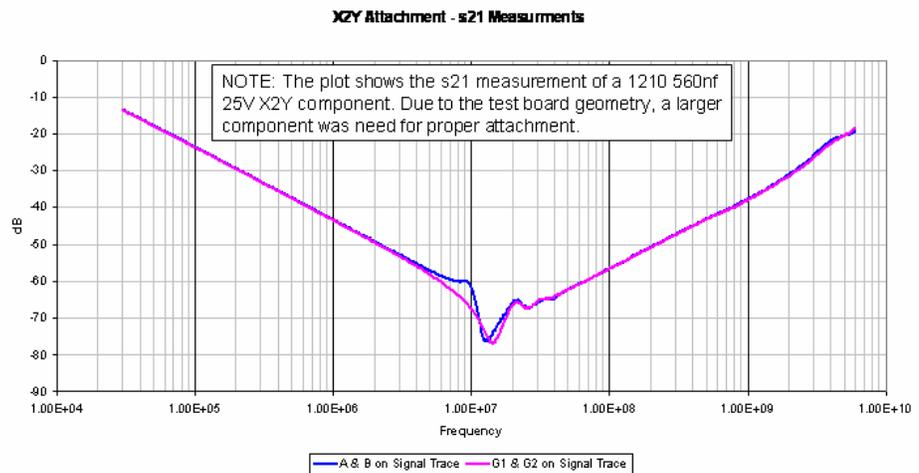
Figure 3. s21 measurements of X2Y® component's attachment in Figure 2.
