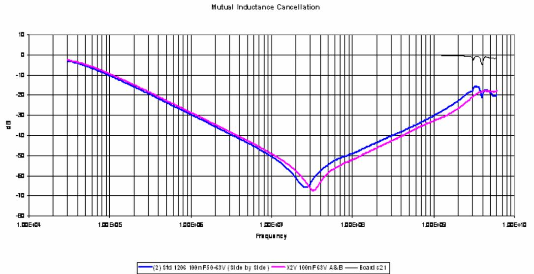
**Figure 7.** s21 measurement results for Test #1 – Flux Cancellation.
