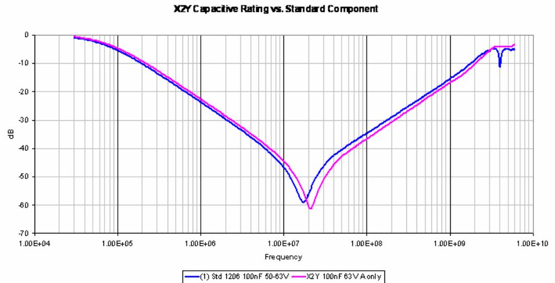
**Figure 4.** s21 measurement of a 100nf standard capacitor vs. 100nf X2Y® component from A to G1/G2 only.
