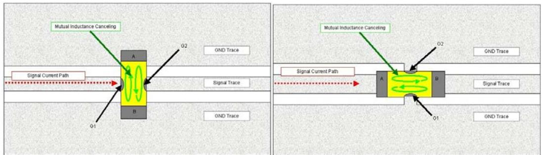
Figure 2. Illustration of X2Y® component PCB attachment for decoupling.
