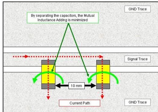
**Figure 8.** Best-case standard capacitor configuration for isolation/separation.
