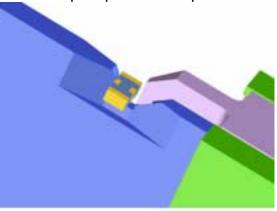
2 DUT guides help place the DUT evenly onto the RF-contacts (DUT guides are shown in blue).
