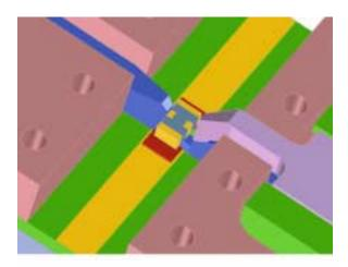
A midsection is inserted into the Test Fixture. The size of the midsection determines the size of the DUT to be tested.
