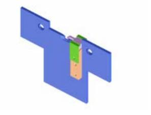
The Midsection has a fixed and a movable ground contact. The movable ground contact slides down a 45 degree ramp. As it slides down, it moves toward the DUT and makes ground contact.
