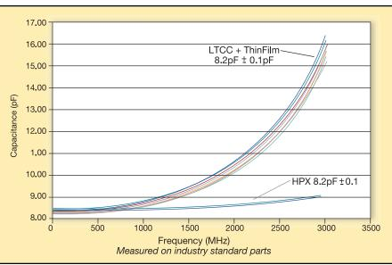
Figure 3. Performance of low temperature, co-fired ceramic (LTCC) vs. discrete high precision capacitor. Courtesy of Vishay Intertechnology.
