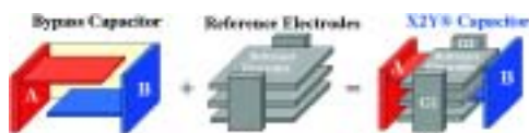
Figure 1. X2Y component's structure is made up of a bypass capacitor in conjunction with reference electrode structure.
