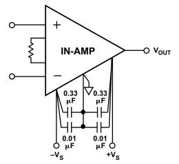
Figure 5-1. Recommended Method for Power Supply Bypassing
