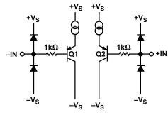
10mA MAX INPUT CURRENT Figure 5-8. AD623 In-Amp Input Circuit
