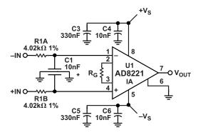
Figure 5-20b. Common-Mode Filter Using X2Y Capacitor
