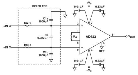
Figure 5-17. AD623 RFI Suppression Circuit
