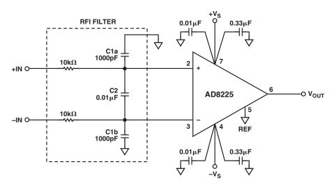
Figure 5-18. AD8225 RFI Filter Circuit
