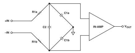
Figure 5-14. Capacitor C2 Shunts C1a/C1b and Very Effectively Reduces AC CMR Errors Due to Component Mismatching
