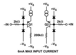
Figure 5-7. AD627 In-Amp Input Circuit
