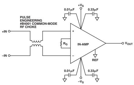
Figure 5-22. Using a Commercial Common-Mode RF Choke for RFI Suppression
