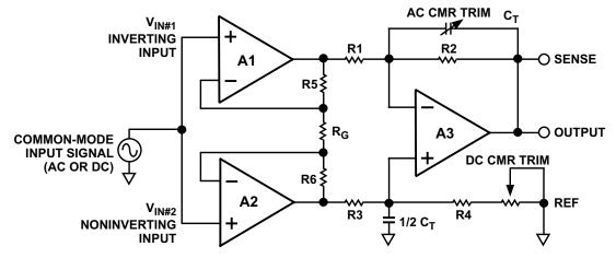
Figure 5-25. External DC and AC CMRR Trim Circuit for a Discrete 3-Op Amp In-Amp
