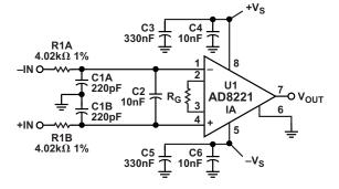
Figure 5-20a. Conventional RC Common-Mode Filter
