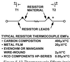
Figure 5-12. Thermocouple Effects Inside Discrete Resistors
