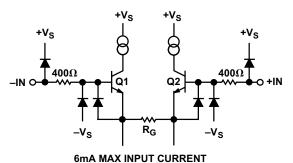
Figure 5-5. AD8221 In-Amp Input Circuit
