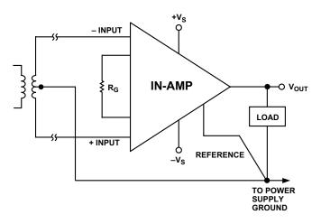
Figure 5-4. Recommended DC Return Path for a Transformer-Coupled Input
