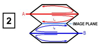
Differential Mode Noise Coupling Note: Differential mode noise cancels at image plane when currents of IA and IB are 180 degrees out of phase
