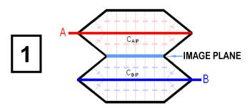
Common Mode Noise Coupling Note: Common mode noise cancels at image plane when capacitors go into self-resonant frequency
