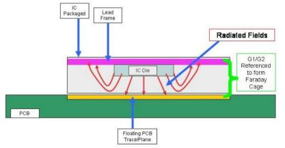
The PCB Trace/Plane and Lead Frame Create a Faraday Cage.
