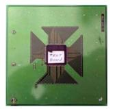
Test Board looking from Inside of TEM-cell
