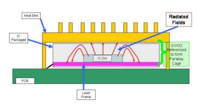
The Heat Sink and Lead Frame Create a Faraday Cage.
