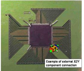
For optimum performance a low-inductance shorting or canceling device should be used between Pwr, GND, and Image Strip. The low-inductive device can be placed internally or externally of the IC package
