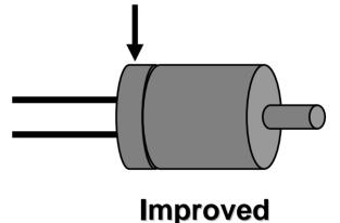
Leads/connector pins should exit the housing close together to reduce current loop.
