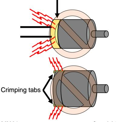
A metal end cap works as a shield to contain the noise within the motor case.
