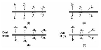
Figure 2. (a) Electric currents and their images in a perfect electric conductor. (b) Magnetic currents and their images in a perfect magnetic conductor. (c) Electric currents and their images in a perfect magnetic conductor. (d) Magnetic currents and their images in a perfect electric conductor.
