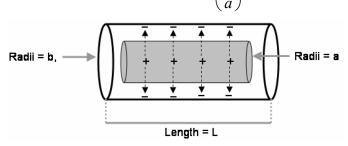
Figure 5. Depiction of a cylindrical capacitor.
