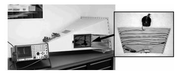
Figure 10. Radiated emissions from a 3 meter cable connected to a washer pump motor were messured in a GTEM.
