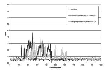
Figure 13. Radiated emissions comparing X2Y<sup>®</sup> inside vs. outside of the washer-pump.
