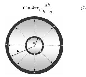
Figure 4. Cross-section of a spherical capacitor.
