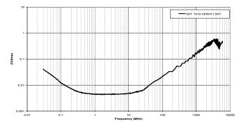
Figure 7. Impedance magnitude plot of a 1410 (400nF) 50v X2Y<sup>®</sup> component in a Circuit 1 configuration.
