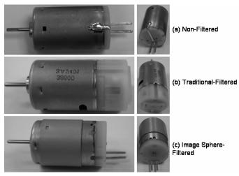
Figure 9. Washer pump motors used as DUTs to measure radiated emissions from power cables.
