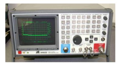
Figure 6. Spectrum analyzer (IFR AN920).
