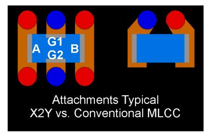
Figure 3. Bypass Capacitor Typical attachments
