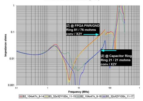
PCB #2 versus #3 100kHz - 300MHz Xilinx test Boards {port 1 to 2}
