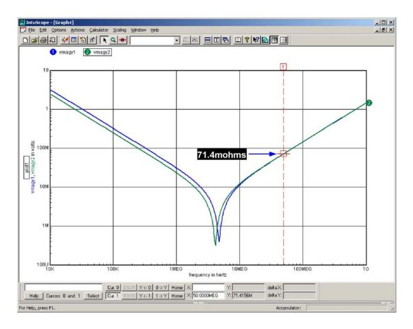
Correlation between the measurement and simulation is reasonable, with actual results for the X2Y array 6% higher than the simulated value, while the conventional capacitor results are some 13% higher. The additional error with conventional capacitors is likely attributable to mutual coupling between the many capacitors in close proximity. The common error is likely due to deviation of the fabricated board stack-up from the model.
