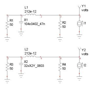
Figure 6. Test Fixture SPICE Model, Simple
