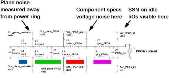
FPGA attachment, plane spreading, and capacitor attachment via inductance all work to decouple the bypass capacitors from the FPGA.
