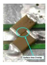
Figure 5. Best-case standard capacitor configuration for cancellation.
